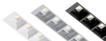
The range consists of four different sizes. Luminaire housing is made of sheet steel, finished with matt white powder coated colour (RAL9003). LED boards are mounted on aluminium heat sink. Extremely quick and reliable fixation into ceilings of different thickness by two strong steel springs. Optical system created by combination of glare eliminating reflectors and highly efficient lenses is designed for premium class office or retail lighting.
