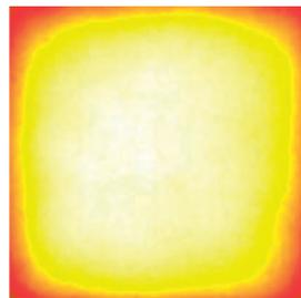
Rotational symmetric light distribution curve with uniform emission of light to all directions allows random orientation of luminaire in space. This unique feature makes it possible to keep the flexibility in interior arrangement.
